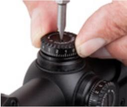
Remove the outer cap. While firmly holding the dial, loosen and remove center screw.
