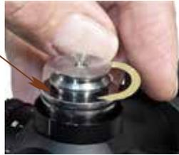
Alternate shim installation direction with each shim.
