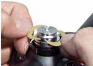
Use as many shims as necessary to completely fill up the space. Do not try to force in a last shim once the clearance is very close—a tiny remaining gap is normal.
