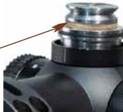
3. After filling the center gap on the post with shims, replace the elevation cap.
