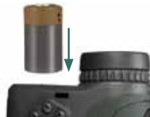
Install battery with positive side facing outwards.
