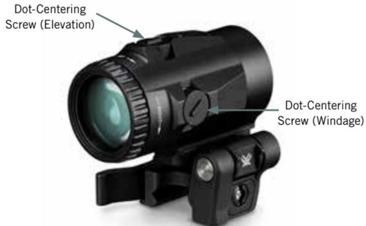
Note: Perfectly centering the red dot in the Micro3X is not required for accuracy. Once the primary red dot sight has been sighted in using its own adjustments, the adjustments done to the Micro3X using the centering screws will not affect the point-of-impact.
