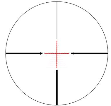
Ultra precision laser etching on the glass reticle ensures that MOA specifications can be kept to the tightest tolerances possible. The fine center crosshair subtensions on the EBR-2B MOA reticle were carefully chosen to provide the optimum balance between precision aiming and low light visibility.
