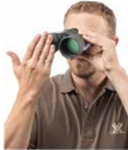
**2. Adjust the diopter**—start by closing your left eye or covering the left objective lens with your hand. Look through your right eye and pull the diopter ring (found on the right eyepiece) toward your eye to unlock and adjust. Rotate the diopter until the object is in focus. Then, push the diopter ring back down to lock your settings. Make note of this diopter setting in case you need to set it again. From this point on, you will only need to use the center focus wheel.
