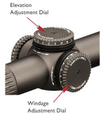
The Razor HD 1-6x24 rifle scope uses clicks scaled in .2 milliradian measurements (MRADs) so each small click will move the point of impact .2 MRADs. **Note:** .2 MRADs equals .72 inches for each 100 yards of distance [2 cm at 100 meters].
