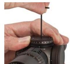
After making this adjustment, the turret cap’s zero mark will correspond with the 200-yard zero on the rifle.
