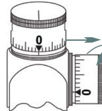
3. Release the dial, allowing it to return to the normal inward position.
