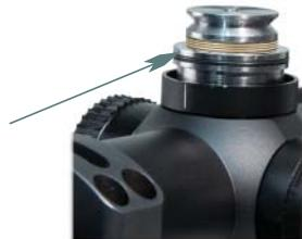
Use as many shims as necessary to completely fill up the space. Do not try to force in a last shim once the clearance is very close.
