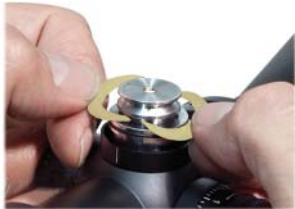
Alternate shim installation direction 180 degrees with each shim.
